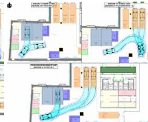
Small Skip Lorry Access and Egress
