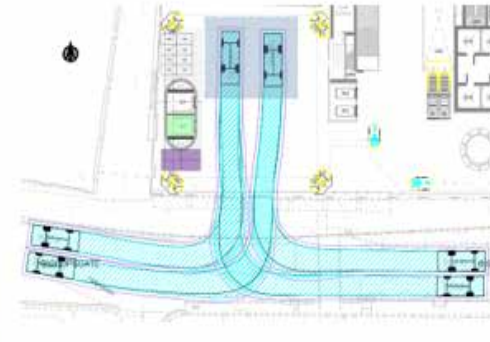
Small Skip Lorry Access and Egress
